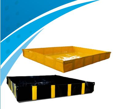
SpillSmart Rigid Bunds provide costeffective temporary storage for liquids and chemicals whilst containing potential spills and leaks. These Bunds are transportable, reusable and ideal for situations where space is minimal. Internal Aluminium brackets insert into specially designed bund pockets, ensuring the 300mm bund walls give great strength, whilst minimising trip hazards and may be removed as required.
