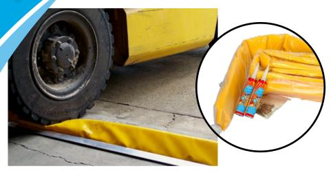
SpillSmart Drive Over Floor Bunding is designed for applications where non-aggressive liquids are being stored and where lower volume forklift or truck access is required. It's constructed with HF welded Heavy Duty 900gsm PVC, encasing high quality 100% memory foam. This combination provides durability and ease of access. The memory foam instantly returns to shape once clear of the vehicle's wheels.
