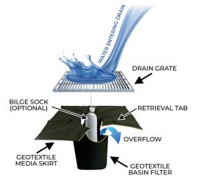
A SpillSmart Drain Warden is an efficient and practical stormwater drain filtration solution for worksites, carparks, marinas and shopping centres.
