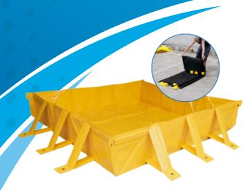
SpillSmart Collapsible Bunds provide costeffective temporary storage for liquids and chemicals whilst containing potential spills and leaks. These Bunds are easy to store and quick to deploy. The external folding legs lock into place keeping the 300mm side walls rigid. Within seconds, the legs can be unlocked and folded down allowing access for pallet jacks, forklifts and vehicles. Eyelets are also provided on the base of the legs if pegging to soft ground is required.
